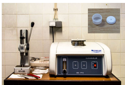
Fig. 2 – Linseis DSC PT-10 and the alumina crucibles used in measurements (top right)
