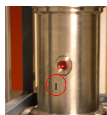
Fig. 3 – General view of the viscosimeter equipment: (A) oscillating initiator connected to the Pt92/W8 suspension wire; (B) He-Ne laser and photo detectors, in a vibration-free table; (C) high temperature furnace; (D) temperature measurement thermocouple; (E) furnace temperature controller; (F) inert gas intake; (G) vacuum system; (H) vibration-free table; (I) quartz window for laser beam; (J) timer interval counter, multimeter and computer for data acquisition and control.
